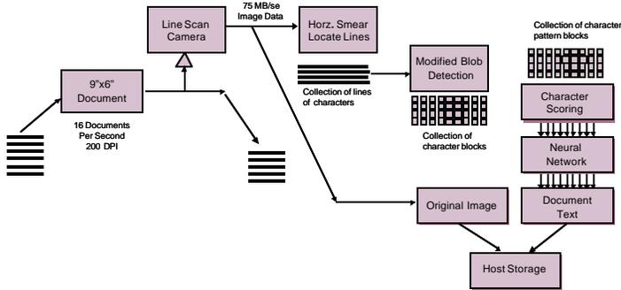
The documents are imaged at 16 per second, or 960 documents per minute, with a line scan camera at 200 pixels per inch. The documents are 9 inches long (parallel to the motion) by 6 inches (perpendicular to the motion or parallel to the camera line).
