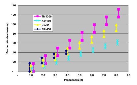
The TM1300 processor also requires two processors to keep up with the image rate, but the cost of the processors (on an auxiliary board in the PC), is significantly less then that of a PIII-450 implementation. The TM1300 product can be obtained for around \$1500 complete, while the multiprocessor PIII system cost several thousand dollars (~\$3000) – more then the basic single processor PC used in the TriMedia solution.
