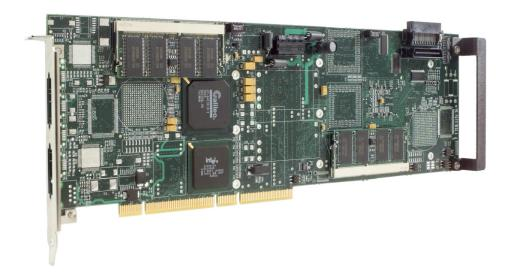
The Basic FastVision is for OEMs who require a framegrabber with high bandwidth data capture. The Basic FastVision is a full-length PCI board with up to 256 MB of dedicated high speed (528 MB/sec) SDRAM. Up to two Channel Link ports are available for data capture. The Basic FastVision board can interface with any high speed Channel Link compatible camera. Applications include medical imaging, semiconductor wafer and mask inspection, wood and PCB Inspection.
