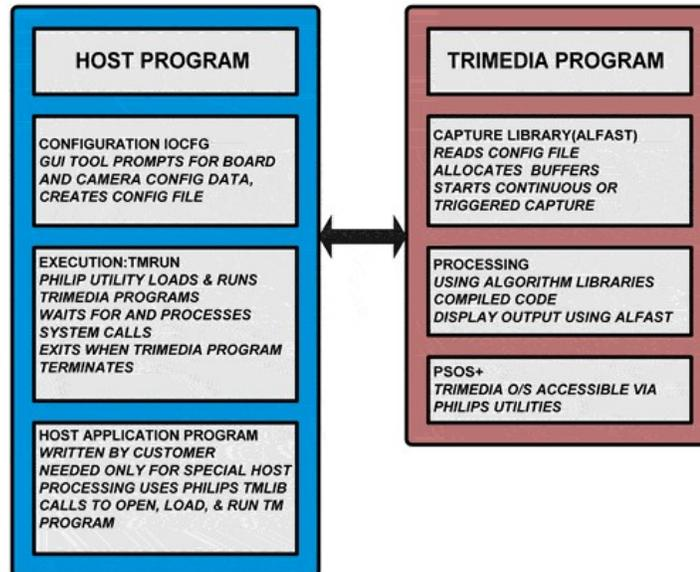
This environment allows the user to use pSOS+ multitasking environment for execution instead of the single tasking ALRT environment.
