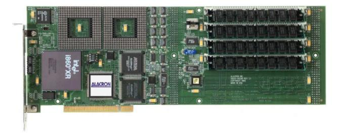
Alacron offers two families of processor boards based on Intel's i860 RISC processors: the AL-860 and FT-200. These boards are ideal for accelerating digital signal processing (DSP), graphics, and imaging processing applications.
