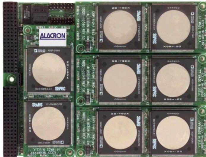
Alacron's FT-2106x-DC deliver high levels of performance for imaging, graphics, simulation, DSP, document processing and pattern recognition applications. The FT-2106x-DC is ideal for adding scaleable compute capability to existing systems, or for developing new systems from the ground up.
