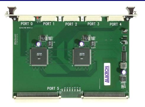
Alacron provides high speed LAN/SAN connections through a combination of PMC and VME interfaces. These boards can be used to build gigabit-per-second System Area Networks (SAN), allowing several computers to work as a system cluster. Individual computers containing the SAN/PMC interface can be linked using the PMC SAN Switch Module.
